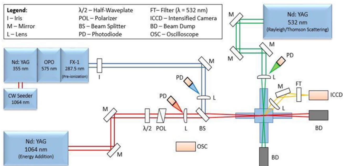
**Figure 7.** Optical layout used for the laser ignition experiments. Dual-pulse REMPI experiments uses overlapped beams from the 287 nm and 1064 nm laser outputs. An additional 532 nm beam is for scattering diagnostics.
