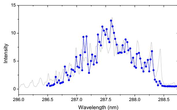
**Figure 2.** Thomson scattering signal from oxygen ( $T = 300$  K,  $P = 1.0$  atm) as function of pre-ionization laser wavelength. Blue symbols and lines are from experiment while the grey line is simulation (see text).
