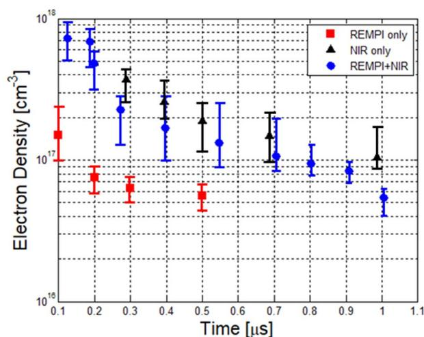
**Figure 3.** Temporal profiles of electron number density after breakdown for three different laser-generated plasmas: O<sub>2</sub> REMPI:  $E_{287\text{ nm}} = 3\text{ mJ}$  (red), single-pulse NIR:  $E_{1064\text{ nm}} = 95\text{ mJ}$  (black) and dual-pulse REMPI:  $E_{287+1064\text{ nm}} = 40\text{ mJ}$  (blue).
