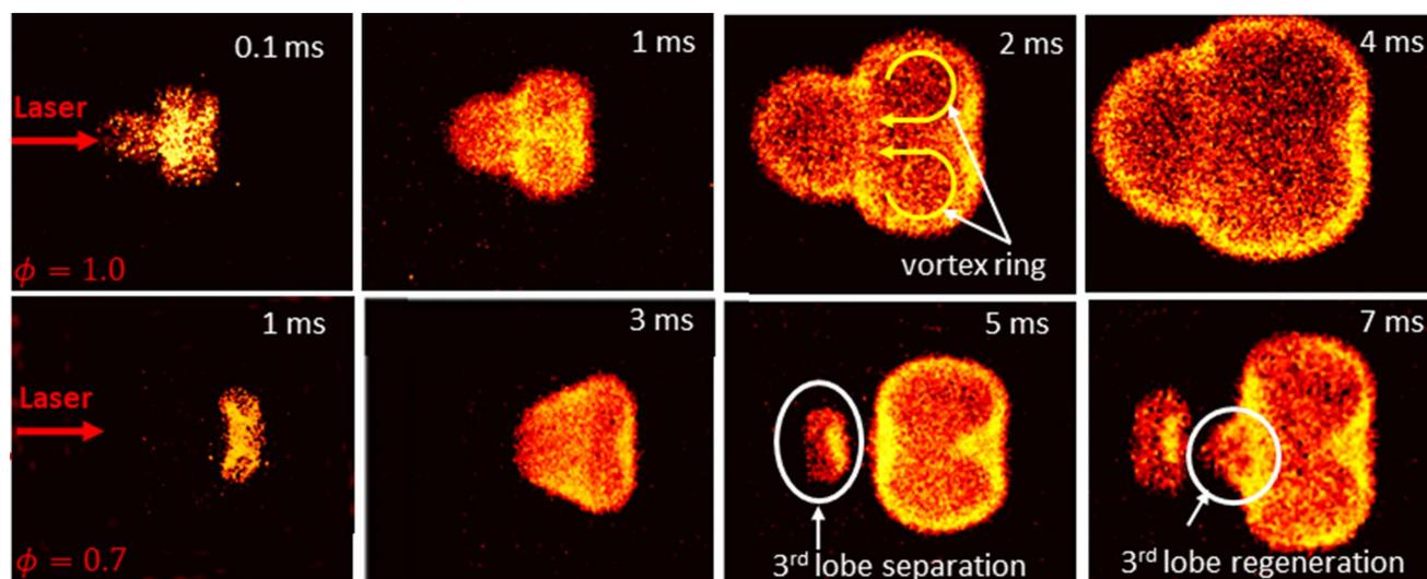
**Figure 6.** OH\* chemiluminescence images showing the early flame kernel dynamics for stoichiometric:  $\phi = 1.0$  (top) and lean:  $\phi = 0.7$  (bottom) mixtures due to laser ignition with the dual-pulse REMPI configuration.
