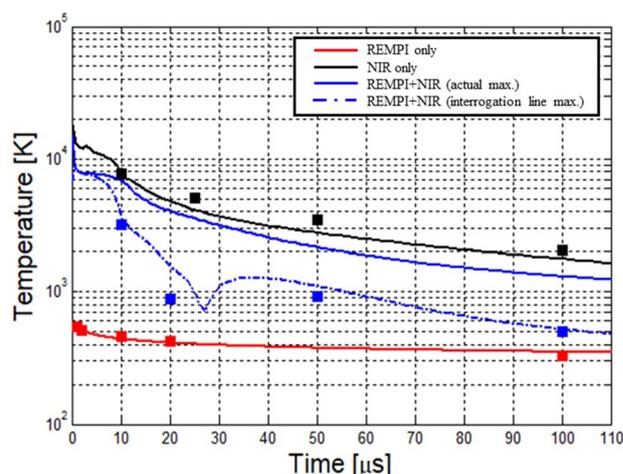
**Figure 4.** Gas temperature as a function of time after breakdown for three different types of laser-generated plasma: 2 + 1 O<sub>2</sub> REMPI (red), NIR (black) and combined REMPI + NIR (blue). Gas temperature profiles predicted by CFD modeling are shown with lines.
