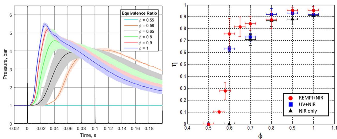
**Figure 5.** Left: Pressure traces due to dual-pulse REMPI ignition of propane–air mixtures. The different curves correspond to different equivalence ratios. Right: Combustion efficiency for 3 cases of laser ignition of propane–air mixtures: dual-pulse REMPI (red), non-resonant dual-pulse (blue), and single-pulse NIR (black). Each point represents the average of at least three tests and the error bars are  $\pm 1$  standard deviation.
