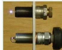
Firing a laser beam through the optical spark plug produces a bigger and more intense spark (top) than a conventional spark plug connected to a high-tension lead (bottom)
