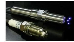
Prototype of a photonic spark plug using Q-switched Nd:YAG:Cr 4+ :YAG microlasers (top), and a standard automobile spark plug (bottom). Photo from Takunori Taira, National Institutes of Natural Sciences, Japan.
