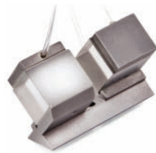
FIGURE 5. This rubidium titanyl phosphate (RTP) Q-switch is assembled in a thermally compensated double-crystal configuration in which two matched crystals are placed in line with the propagation axis with one crystal rotated by 90° with respect to the other. (Image credit: Raicol Crystals)
