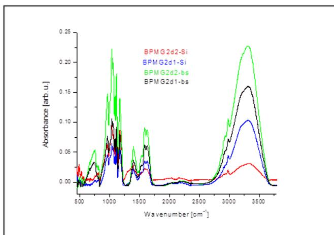
Fig. 10a) FTIR spectra of sol-gel thin films on Si and borosilicate glass - BS, dried at 120°C
