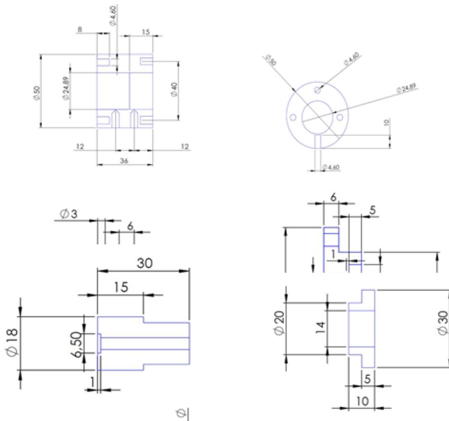
Fig. 26. Technical drawings for Faraday isolator Model 2
