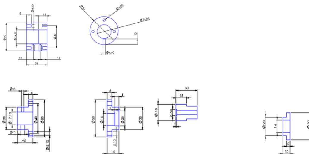
Fig. 25. Technical drawings for Faraday isolator Model 1
