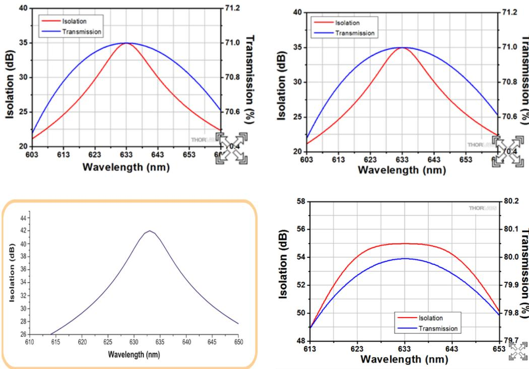
Fig. 23. Main technical features of Faraday rotator for 633 nm, wavelength depending of polarization.
