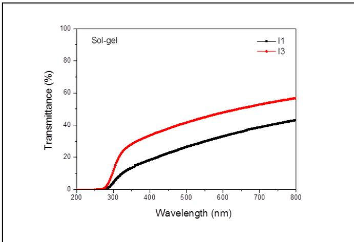
Fig. 18a) UV-VIS Transmittance of films BPM6-2d1 (I1) and film BPM6-2d2 (I3), obtained by sol-gel, deposited on borosilicate glass
