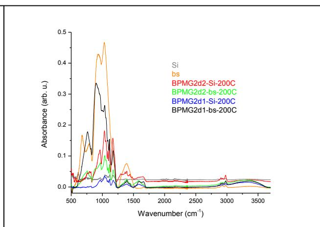
Fig. 10b) FTIR spectra of sol-gel thin films on Si and BS, treated at 200°C and of substrates
