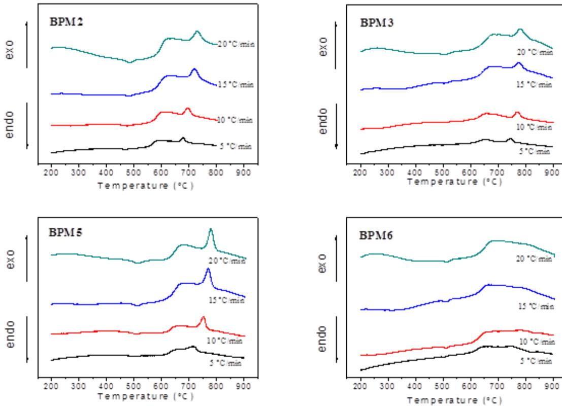
Fig. 13. DSC results at different heating rate
