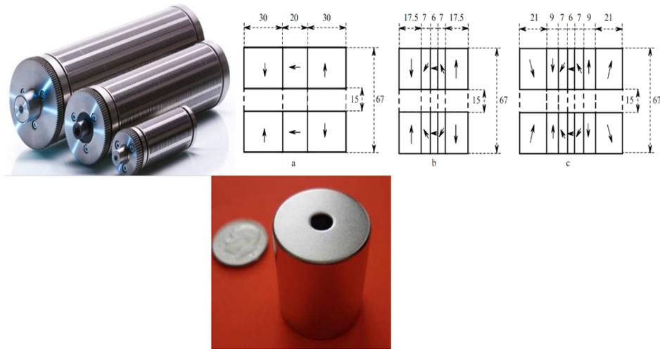
Fig. 21. Optimal dimensions of cylindrical magnet for an optical isolator with radial opening of 12mm with rings of magnetic field a) radial and axial. B) Imagnetization rings, axial and sidelong All dimesnsions are in mm
