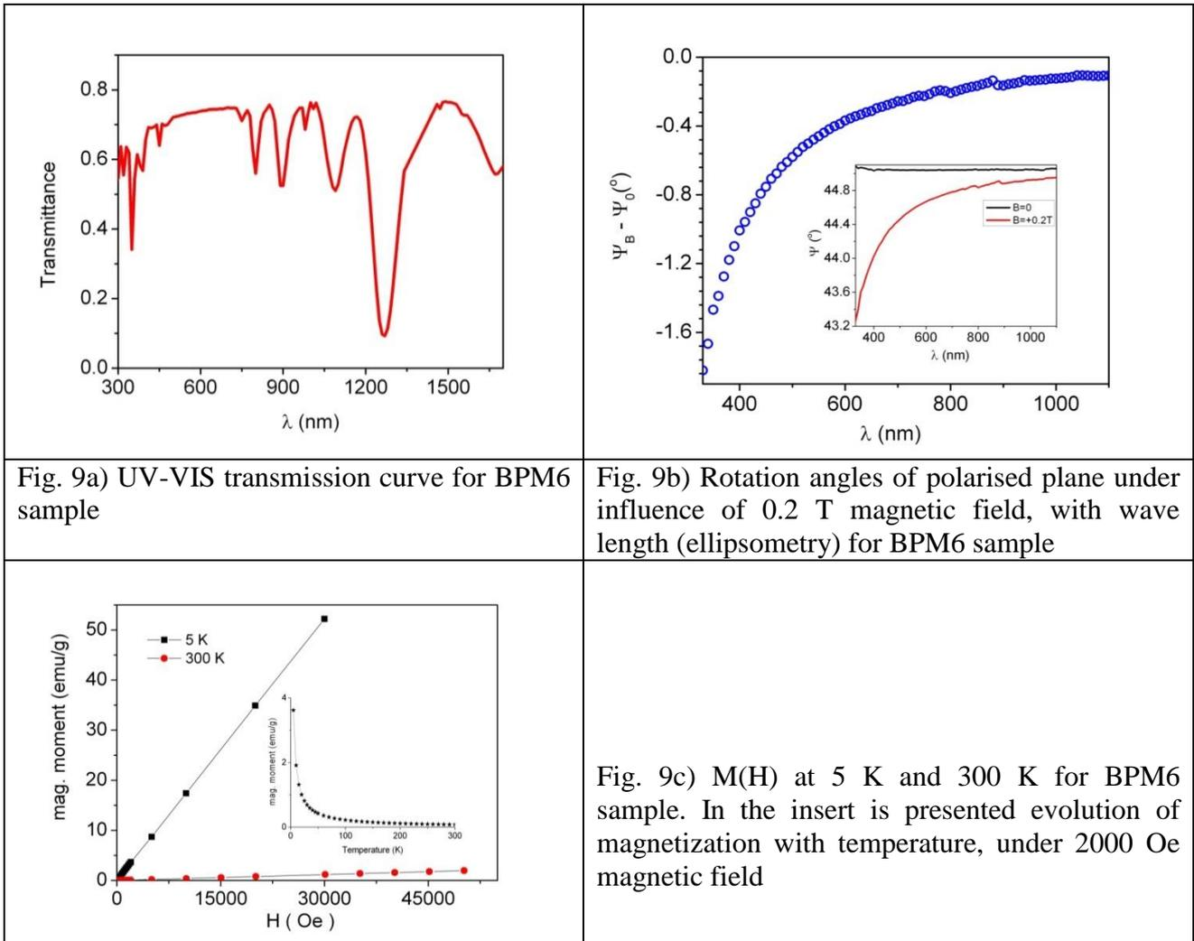
At wavelength of 600 nm, Verdet constant for BPM6 samples is about 0,06 min/mm/Oe, and a rotation of 5 min with a glass of 1 cm length is obtained in a field of 90-100 Oe. BPM6 sample depass 3 times the BMP2 sample.
