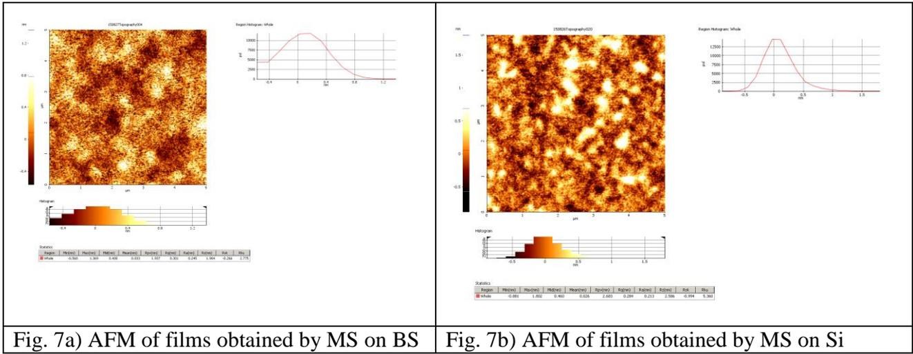
It was identified that the films have the same composition as the glass target. Films with 0.5-1 microns thickness were obtained by magnetron sputtering deposition from boro-phosphate glass target. The films were smooth as the AFM showed out.
