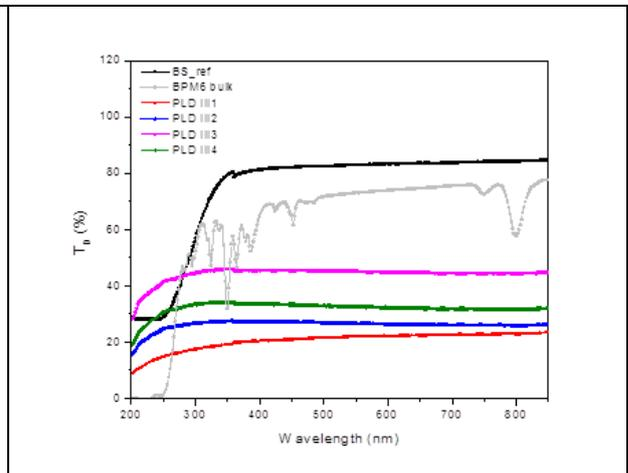
Fig. 18b) UV-VIS Transmittance of the films BPM6\_III1 to III4 obtained by PLD and deposited on BS glass substrate. Comparison of values obtained for BPM6 bulk and BS substrate is shown
