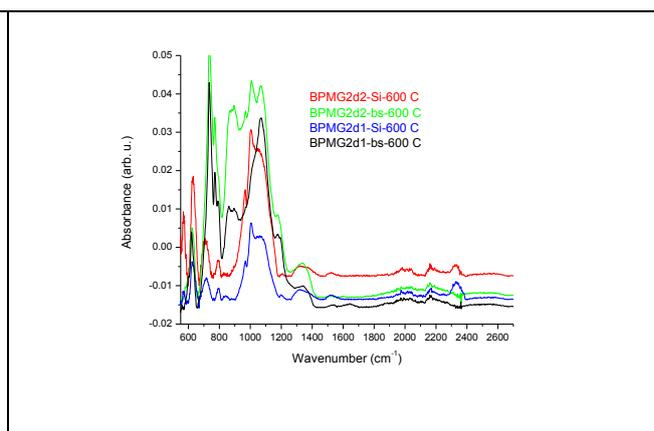
Fig. 10d) FTIR spectra of sol-gel thin films on Si and BS, treated at 600°C
