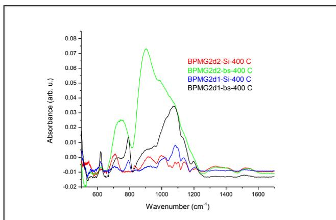
Fig. 10c) FTIR spectra of sol-gel thin films on Si and BS, treated at 400°C
